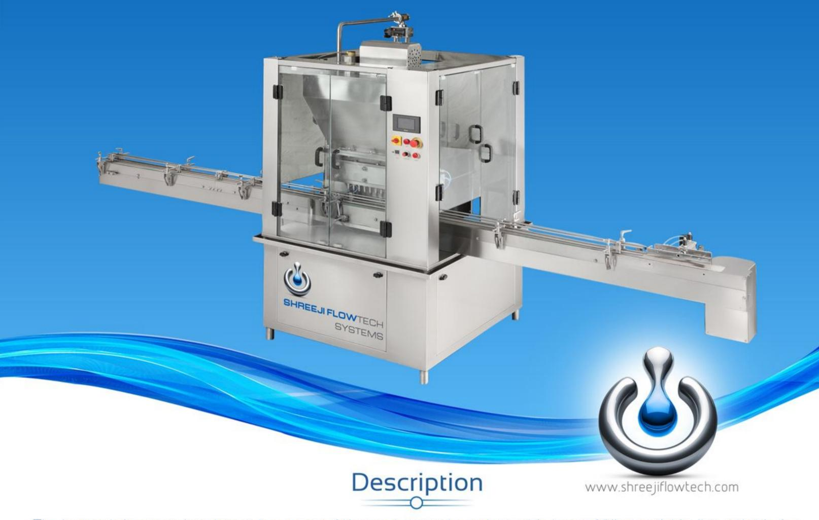
The horizontal servo volumetric piston is one of the most accurate and versatile type of filler available. It is suitable for handling a wide variety of semi-viscous and High Viscous products.
