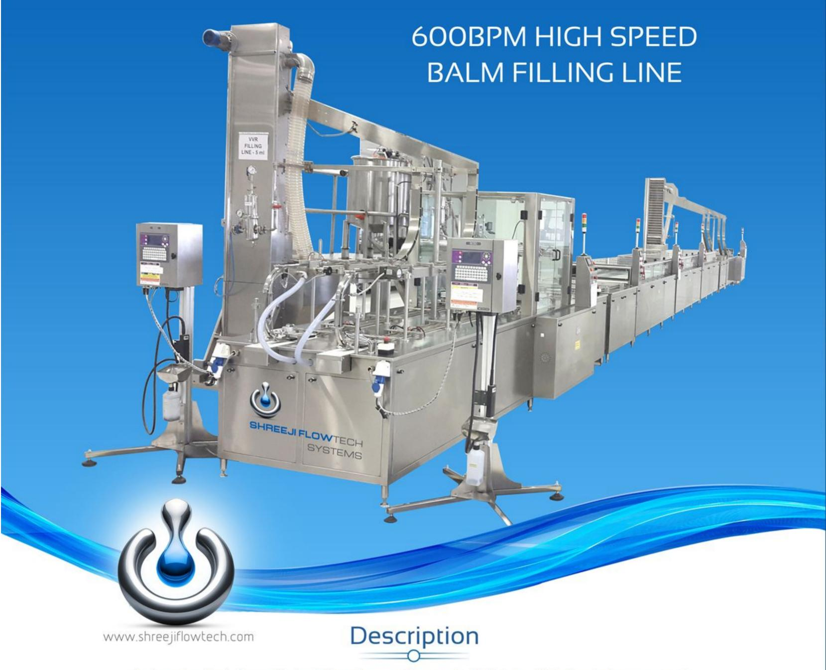
Automatic High Speed Balm Filling Line with speed of 400 to 600 Products per minute Line consisting of Empty Tub/Dibbi Feeding having built in Airjet Blowing/Cleaning, Filling, cooling and Capping System.
